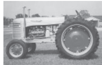
Richard Lyman restored this 1955 Silver King tractor, built in West Virginia, with a Ford flathead V-8 100 hp engine.
