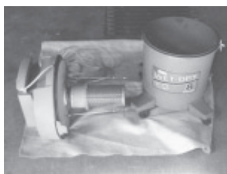
Lowell Blakely adapted an old air filter from his skid loader to fit his Sears shop vac.
